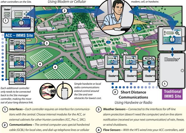
station level diagnostics and real-time flow monitoring!
