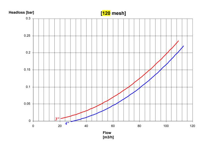
\* Flow rate data is for high quality water at a filtration grade of 200 micron.
